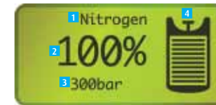
1 Gas type 2 Remaining quantity of gas in percent 3 Inlet pressure 4 Indication of the remaining gas contents
