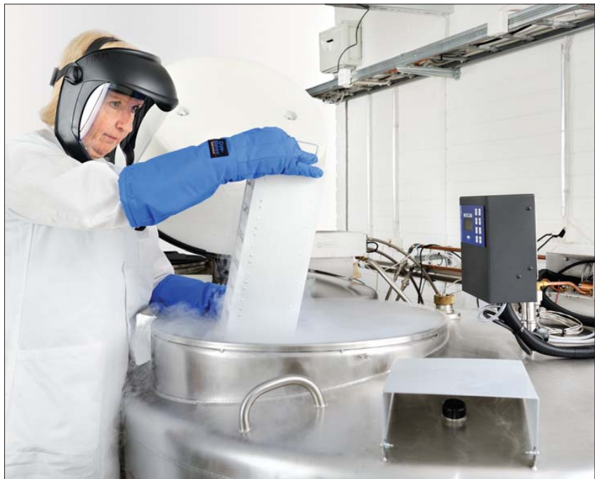
Liquid nitrogen can be used to store biological samples indefinitely, without risk of degradation, at temperatures as low as -196 degrees C.
