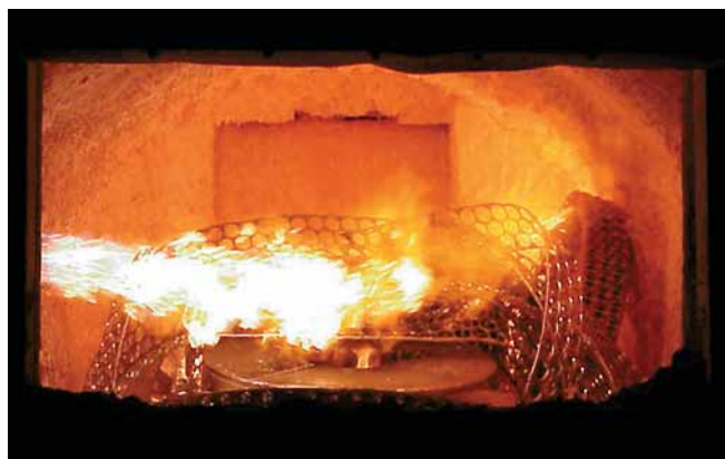
Oxyfuel burner in a reverberatory melting furnace
