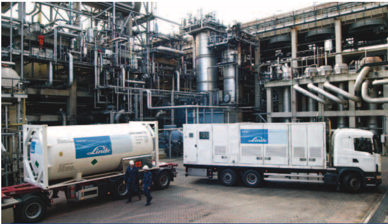
Figure 2. An effective method to recover solvent vapours is to condense and capture them using liquid nitrogen.
