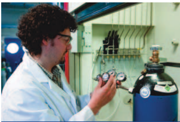
Figure 1. High quality gas control equipment is essential to deliver high purity gases to the GC-MS instrument.
