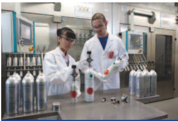
Figure 3. Linde HiQ specialty gases come in highly portable cylinders for calibration of remotely located lower explosive limit and lower flammable limit sensors.
