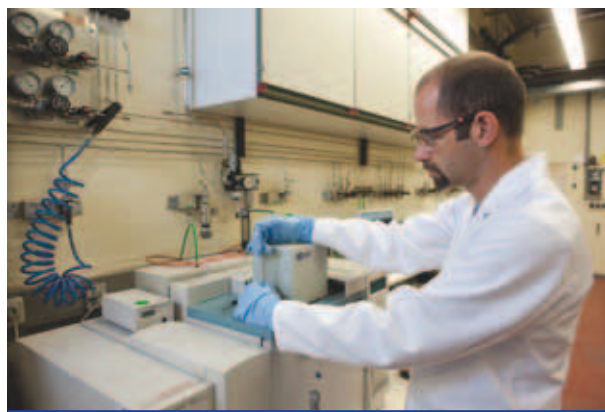
Figure 2. GC-MS separates components and analyses in the gaseous phase, in addition to some samples that normally exist in the liquid phase.
