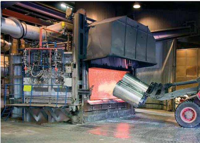
Low-temperature oxyfuel combustion is used to increase melting capacity, reduce dross and achieve ultra-low NOx emissions at Sapa Heat Transfer AB (Elkem Group) in Sweden
