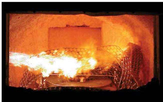
Oxyfuel burner in a reverberatory melting furnace
