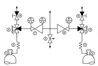
1 GAS CYLINDER 2 COIL/ HOSE 3 SHUT-OFF VALVE (3XIN; 1XOUT) 4 PURGE OUTLET VALVE 5 RELIEF VALVE 6 FIX PRESSURE REGULATOR 7 SET PRESSURE REGULATOR A 300 – 14 bar
