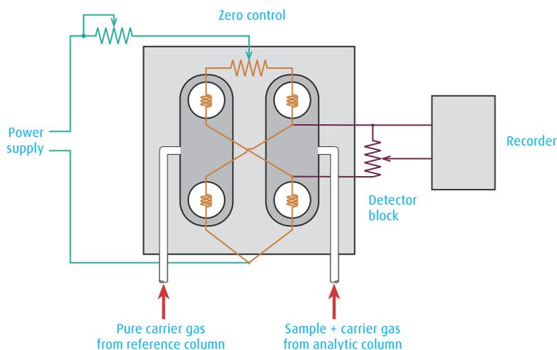
Chemically active compounds like acids and halogenated compounds should be avoided when using TCD since they can attack the filament (wires) and thereby change the resistance and permanently reduce the detector sensitivity. Oxidizing substances, such as oxygen, can also damage the filament, and a leak free environment should be maintained.
